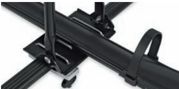
Fixing on the bars by means of U-bolt or with "T" insert (included). Fissaggio con cavallotto o con inserto a "T" incluso.
